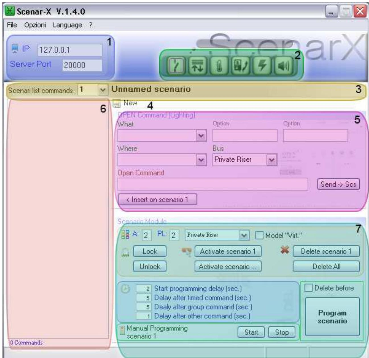
**Fig. 1/1** : Address and local port setting to communicate with the web server.
