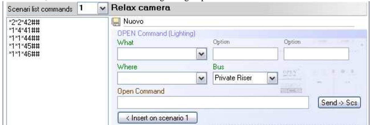
NB: Open commands have two optional boxes, both must be completed or open or an optional part will not be generated.
